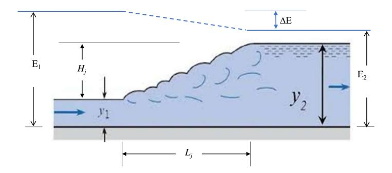
*Example:* Water flow through of flume with a depth of (0.6 m), and unit discharge (q) of (3.7 m3/sec/m). Does a hydraulic jump occur or not? Determine the depth of flow at the D/S of the jump and find the energy dissipation for this jump ( $\Delta E$ )
