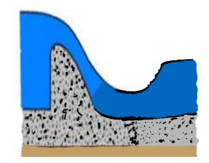
A still basin is a short length of a paved channel placed at the end of any supercritical flow. The aim of the designs is to make a hydraulic jump form within the basin, so that the flow is converted to subcritical before it reaches the exposed and unpaved riverbed at D/S.
