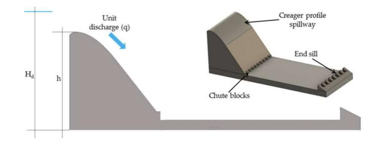
The chute blocks, located at the entrance to the stilling basin, serve to increase the effective depth of the entering stream, break the stream up into a number of small jets, and help create the turbulence required for effective energy dissipation.
